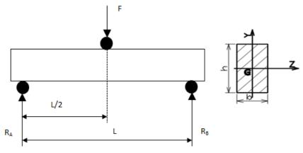
Figure 4: 3 point bending test
