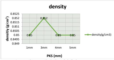
Figure 7: densities of palm kernel shell-plastic composites
