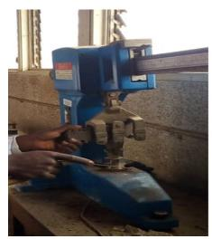
Figure 5: flexural testing machine
