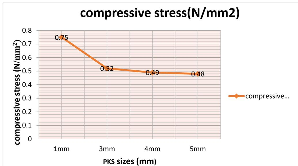
Figure 6: compressive strength vs. PKS sizes
