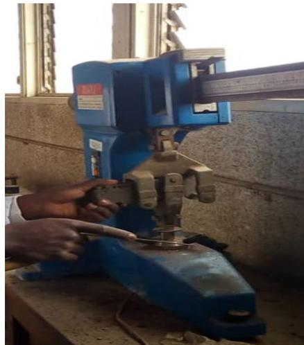
Figure 5: flexural testing machine
