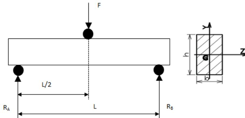
Figure 4: 3 point bending test
