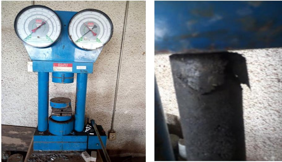
Figure 3: Specimen on compressive load and failure
