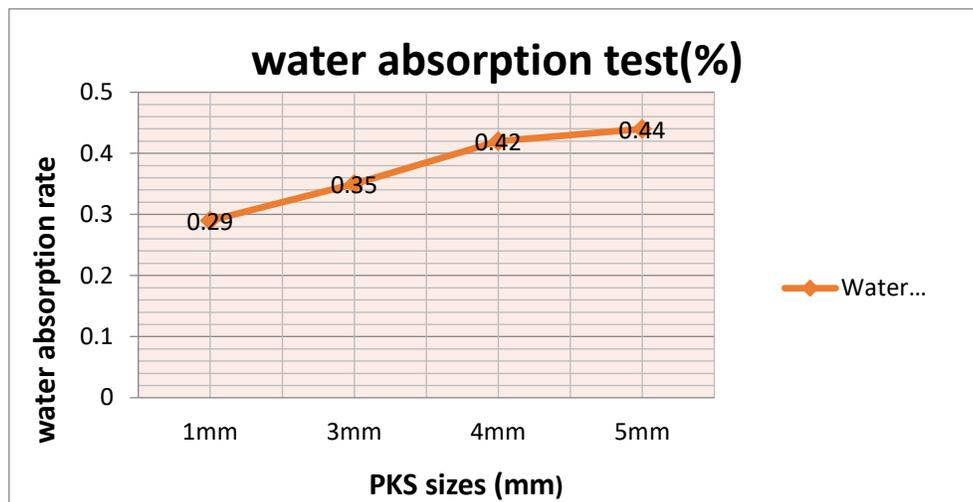
Figure 9: Plot of water absorption rate against the PKS size
