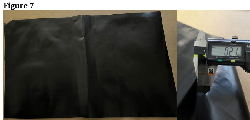
Figure 7 Conductor Film from Calendering Process (Left), Film Thickness Measurement (Right)
