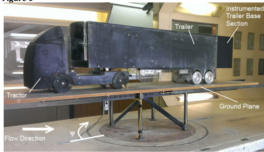
Figure 1 Wind Tunnel Test Setup with Instrument Base, Re_n = 8 \times 10^5
