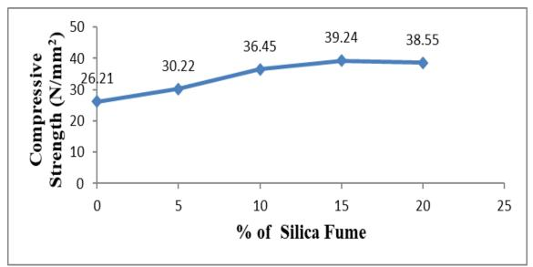
**Figure 8:** Results of Compressive Strength (7 days)
