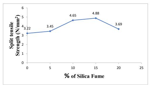
Figure 10: Results of Split tensile Strength (7 days)
