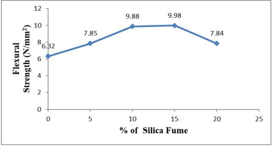
Figure 13: Results of Flexural Strength (28 days)
