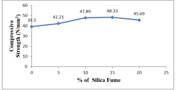
**Figure 9:** Results of Compressive Strength (28 days)
