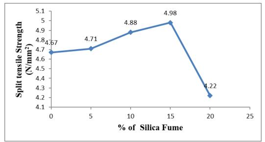
Figure 11: Results of Split tensile Strength (28 days)
