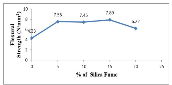
Figure 12: Results of Flexural Strength (7 days)
