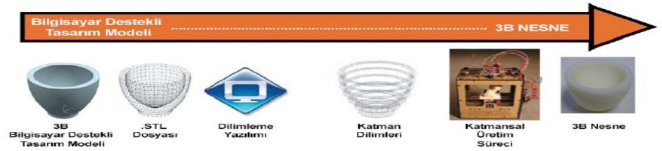
**Figure 1** Additive Manufacturing Process [Campbell et al. \(2011\)](#)
