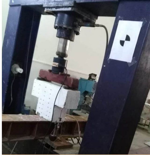
Figure 5 The Hydraulic Machine for Testing Concrete Piers
