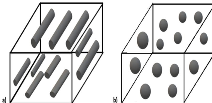
**Figure 9** Composite materials a) matrix with continuous fiber reinforcement, b) matrix with particle reinforcement
