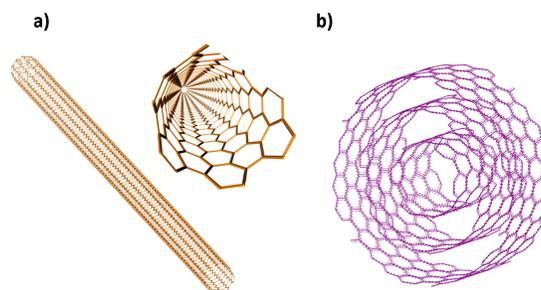
**Figure 10** Carbon nanotubes: a) Single-walled carbon nanotubes and b) Multi-walled carbon nanotubes.
