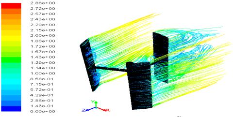
Figure 2: Simulation of Darrieus Turbine<sup>1)</sup>
