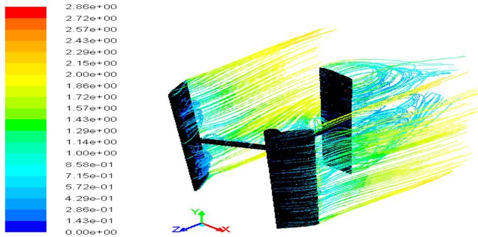
Figure 2: Simulation of Darrieus Turbine<sup>1)</sup>
