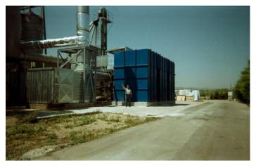
Figure 1: The three bed thermal regenerative oxidizer plant in Lecheum-Corinth operated by ZOONOMI SA
