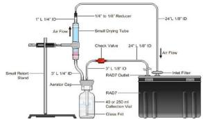
Figure 3: Schematic Diagram of RAD7 Detector with RAD H<sub>2</sub>0 Accessories.
