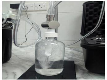
Figure 5: Aeration stage during radon measurement
