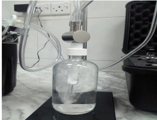
Figure 5: Aeration stage during radon measurement
