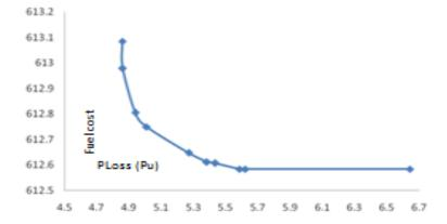
Figure 5: Pareto optimal graph between Ploss Fuel cost
