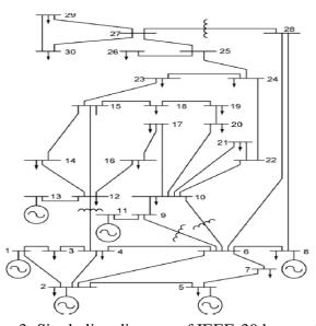
Figure 3: Single line diagram of IEEE-30 bus system
