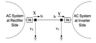
Figure 2: main structural diagram of HVDC line
