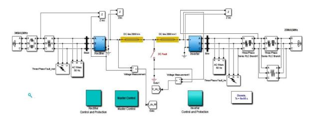
HVDC 12-pulse Transmission System 1000 MW (500kV-2kA) Fig 9 MATLAB/Simulink model of HVDC line
