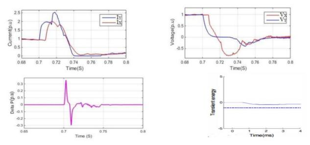
Figure 10: simulation result on inverter side of external fault
