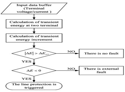
Figure 8: traveling wave algorithm for transient energy
