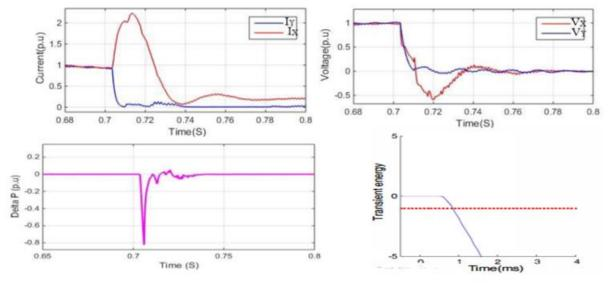
Figure 12: simulation result of HVDC line on an internal fault
