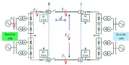
Figure 1: main components of HVDC transmission line
