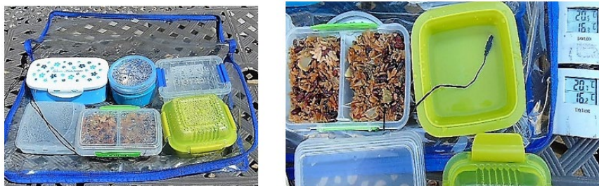
Figure 9 Heating of 6 lunch boxes in plastic bag, with pinto and water temperature sensors
