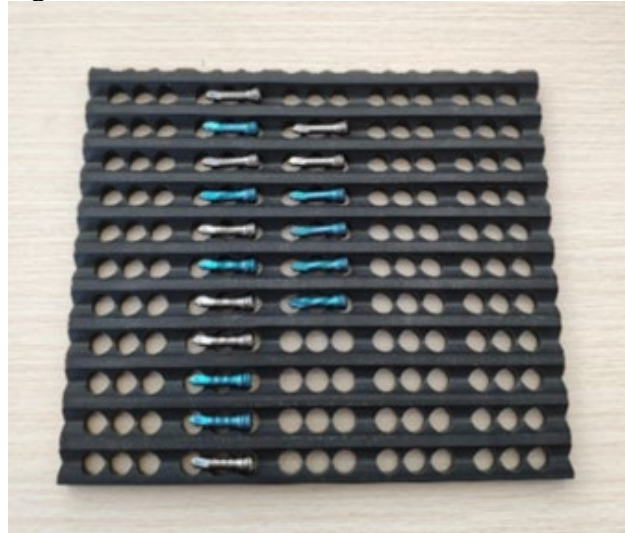
Figure 3 Tooling Fixture for Bone Nails
