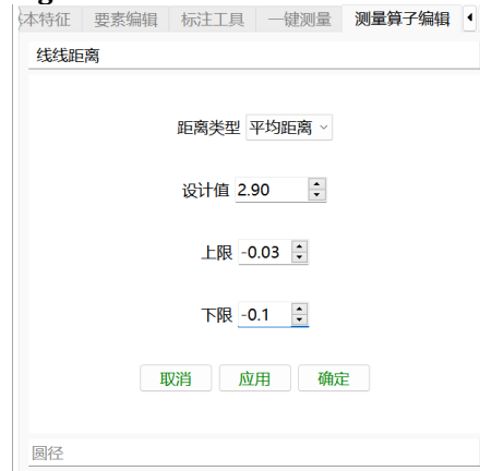
Figure 10 Tolerance Setting Interface
