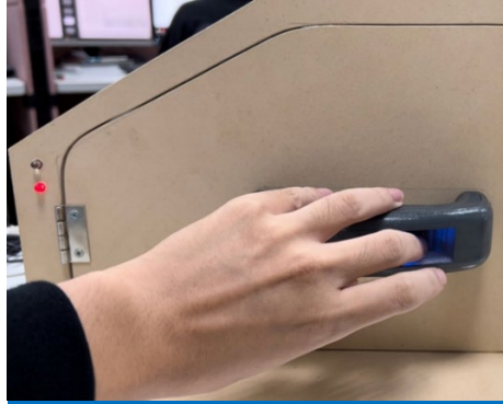
Figure 9 Red Light Turns on when Fingerprint is not Correct
