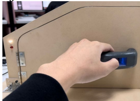
Figure 8 White Light Turns on When Fingerprint is Correct
