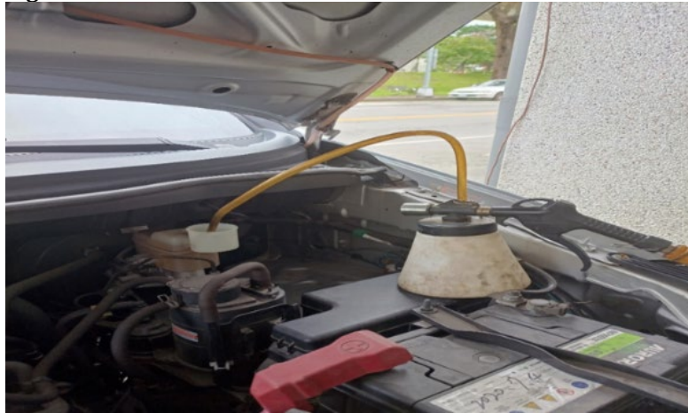
Figure 2 Brake Fluid Samples Taken from Real Vehicles
