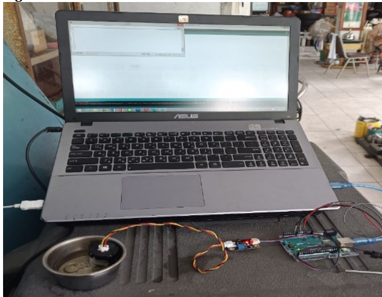
Figure 3 Measuring the Brake Fluid Turbidity and Water Content
