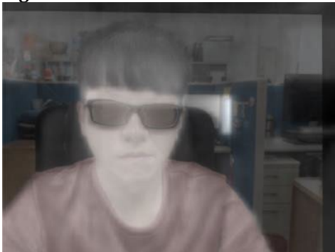
Figure 13 Thermal Image and Visible Image Superimposed after Homography
