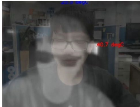
Figure 12 Thermal Image and Visible Image Superimposed Before Homography
