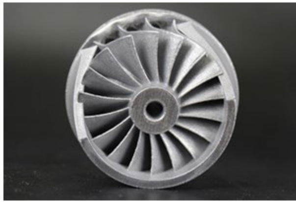
Figure 8 An impeller made from ultra-porous binder jetting powders by Uniformity labs and Desktop metal Additive Manufacturing (2022)
