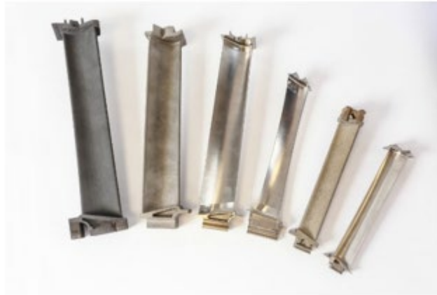
Figure 2 3d printed turbine blades made using SLM for aerospace applications by Avio-Aero Kellner (2018)
