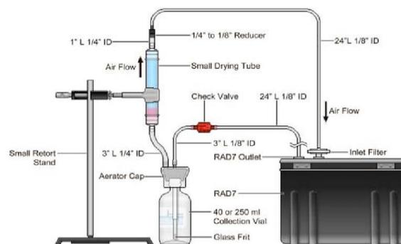
Figure 3: Schematic Diagram of RAD7 Detector with RAD H<sub>2</sub>O Accessories.
