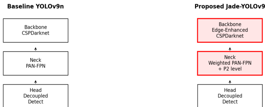
Figure 1 Baseline YOLOv9n and the Proposed Jade-YOLOv9 Architecture. Red Blocks Indicate Modified Components
