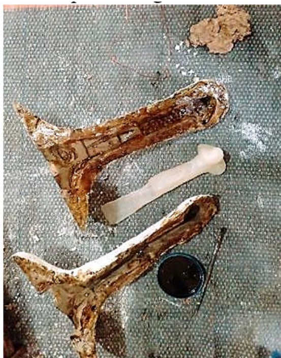
Figure 14 Separation of the Mother Mold, Oiled and Ready for Positive Cast Medium: POP, Silicon, Clay. Milled Steel Rod, And Twisted Wire Year: 2026 Artist: Ephraim Ugochukwu
