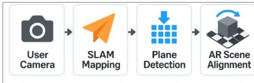
Figure 6 Scene Assembly Process Showing Slam-Based Spatial Mapping and Real-Virtual Content Alignment
