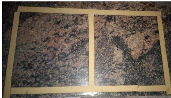
Figure 2 Mould made from rectangular plywood
