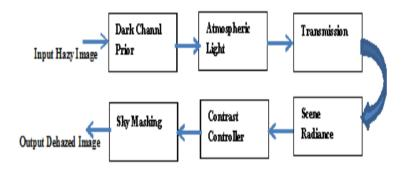
Figure 4 shows the methodical steps to develop the code. At first, the low-intensity pixels are measured by turning the fuzzy picture into a black channel. From the dark channel, the atmospheric light is then computed. The next step is to transform the input picture into RGB and then into HSV (Hue Saturation Value). One last step involves applying filters to the hazy picture using the scene depth values that are connected with the derived parameters.
