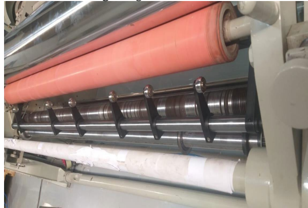
Fig 10: Development of modified paper rewinding machine paper support system
