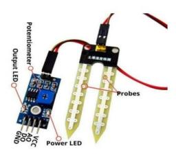
Figure: Soil Moisture Sensor
