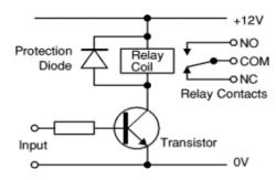
Fig: Relay Operation and use of protection diodes
