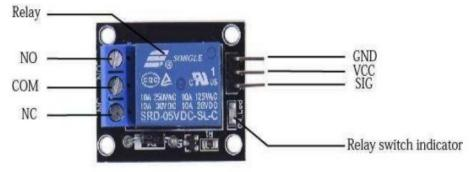
Figure: Pins of Relay
