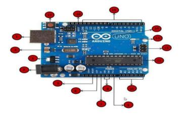
Figure: Arduino uno board
