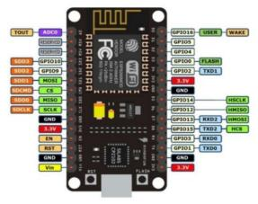
Figure: Pin Diagram of Node MCU
