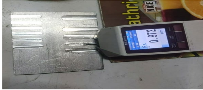
Fig 2. Talysurf instrument for measuring surface roughness
