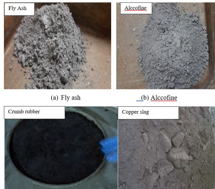
Figure 1 Physical images of fly ash, alccofine, crumb rubber and copper slag aggregates.
