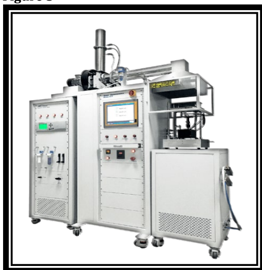
Figure 3 Cone Calorimeter Test (ISO 5660)
