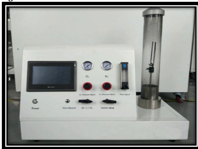
Figure 2 Limiting Oxygen Index (LOI) Test (ASTM D2863)
